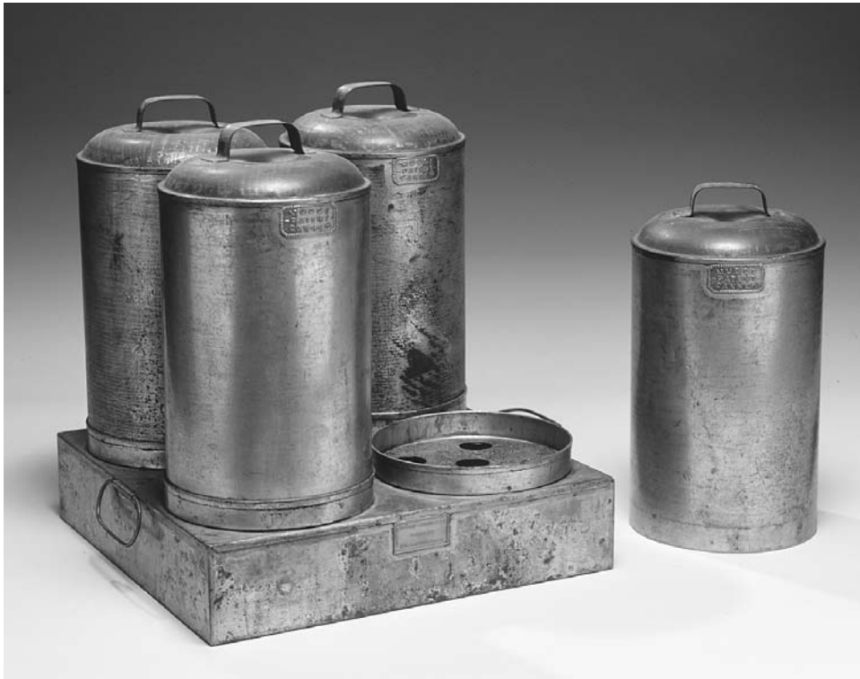
The introduction of the kitchen range brought about a revolution in home canning and preserving. The Mudge Stovetop Canner (shown here) was introduced in the early 1900s as a tool for sealing jars. Glass jars were placed inside the tight-fitting metal containers. Boiling water in the base caused steam, which built up pressure and thus sealed the jars. ROUGHWOOD COLLECTION. PHOTO CHEW & COMPANY.
